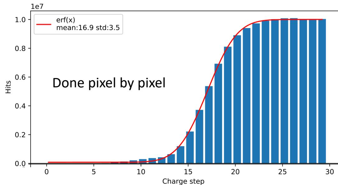
In-pixel charge injection to measure the comparator threshold
