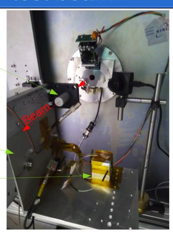
PD package was never positioned in a cube face perpendicular to te beam direction
