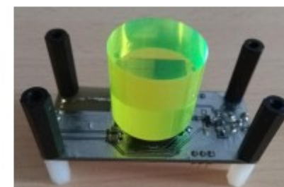
SiPM preamplifier board with EJ-276G scintillator
