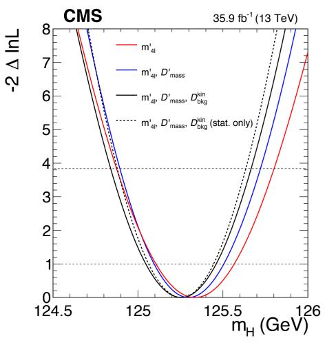
A mass constraint on the intermediate on-shell Z resonance has been exploited in order to improve m<sub>#</sub> resolution
