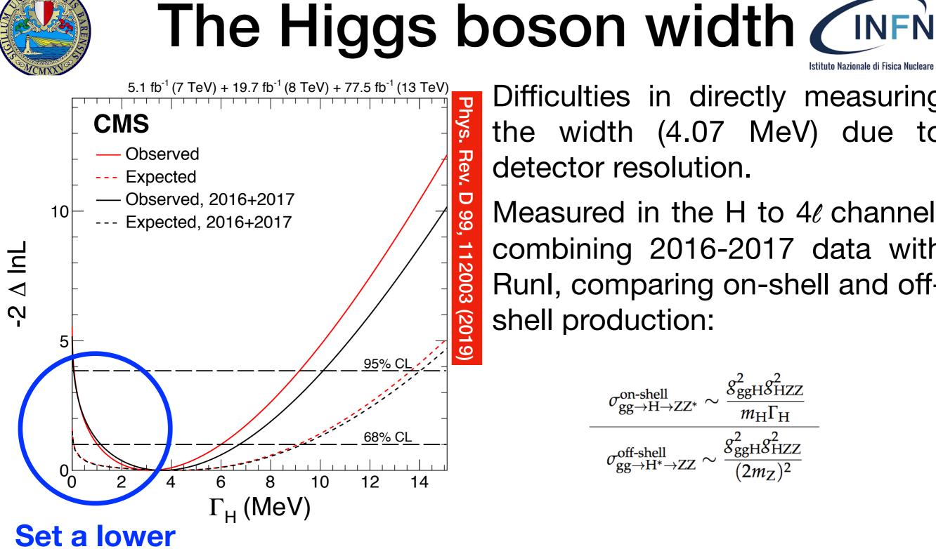
Difficulties in directly measuring the width (4.07 MeV) due to detector resolution.
