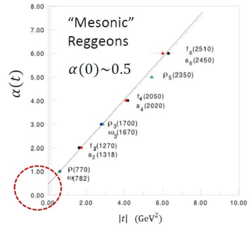
All Reggeons corresponding to known mesons exchange have intercept below 1  $\rightarrow$  Pomeron ( $C=P=1$ ) introduced as the dominant trajectory with intercept above 1 to explain the observed increases with energy of hadronic cross sections
