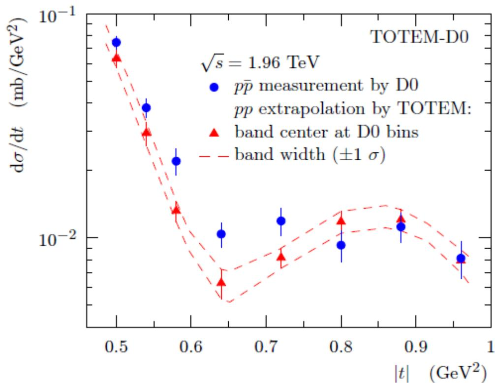
$\chi^2$  test to examine the probability for the D0 and TOTEM differential elastic cross sections to agree.
