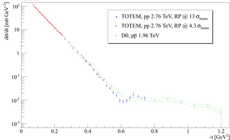
Dip-bump structure compared with the Do published results. Main parameters:
