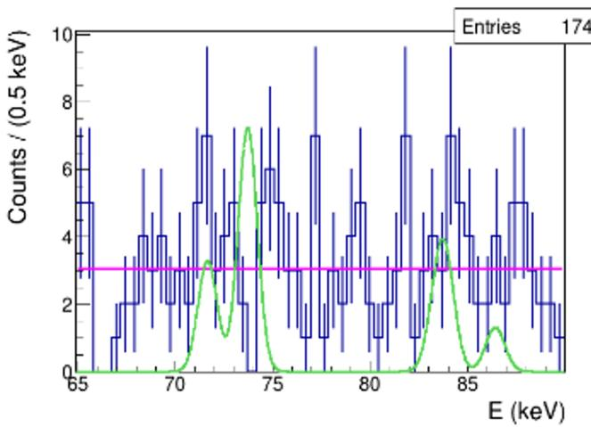
FIG. 1. The measured X-ray spectrum, in the region of the  $K_{\alpha}$  and  $K_{\beta}$  standard and violating transitions in Pb, is shown in blue; the magenta line represents the fit of the background distribution. The green line corresponds to the shape of the expected signal distribution (with arbitrary normalization) for the  $A_3$  analysis and the  $M_3$  parametrization.
