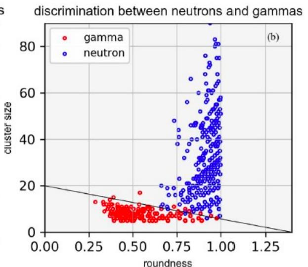
For a selected track,  $CV$  is the sum of the ToT counts on all the pixels belonging to the track,  $CS$  is the total number of pixels in a track. The  $CR$  parameter, instead, is defined as the ratio between the diameter of the circumference having the same cluster area and the length separating the two most distant pixels in the cluster [16].
