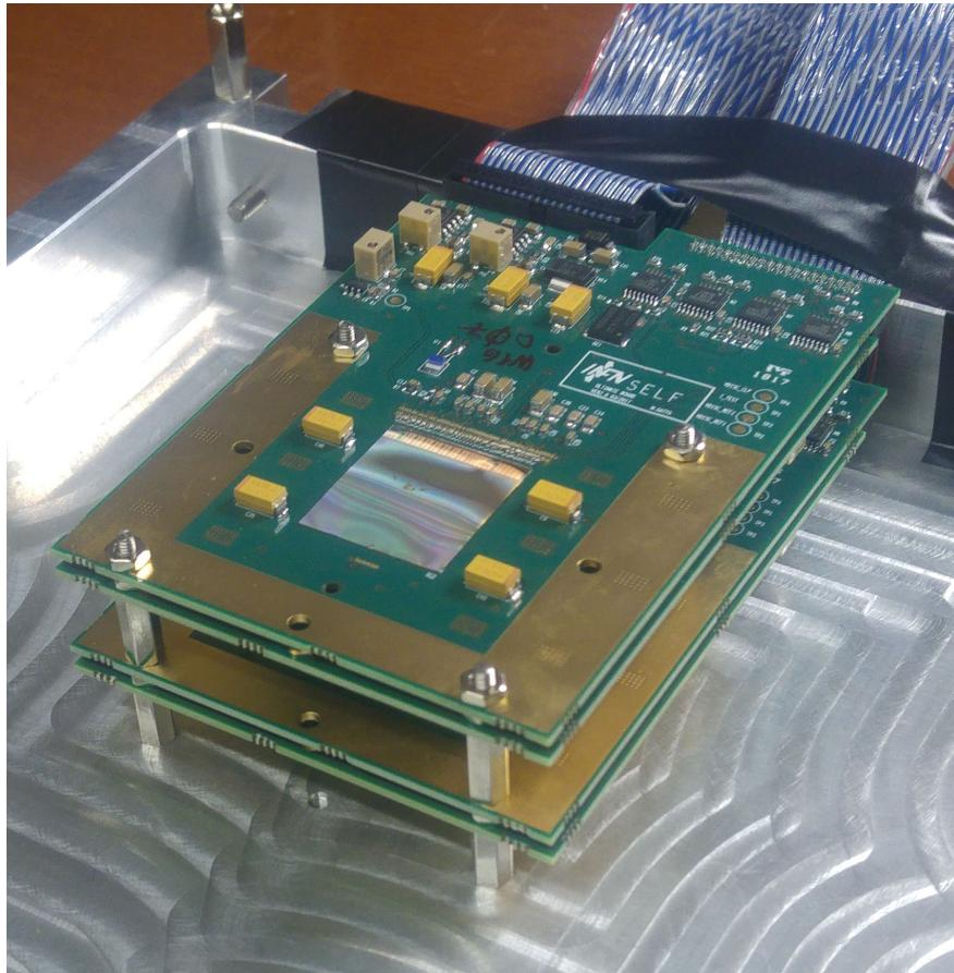
**Pixel Vertex: 4 planes of M28 sensor, 50 $\mu$ m thick**
