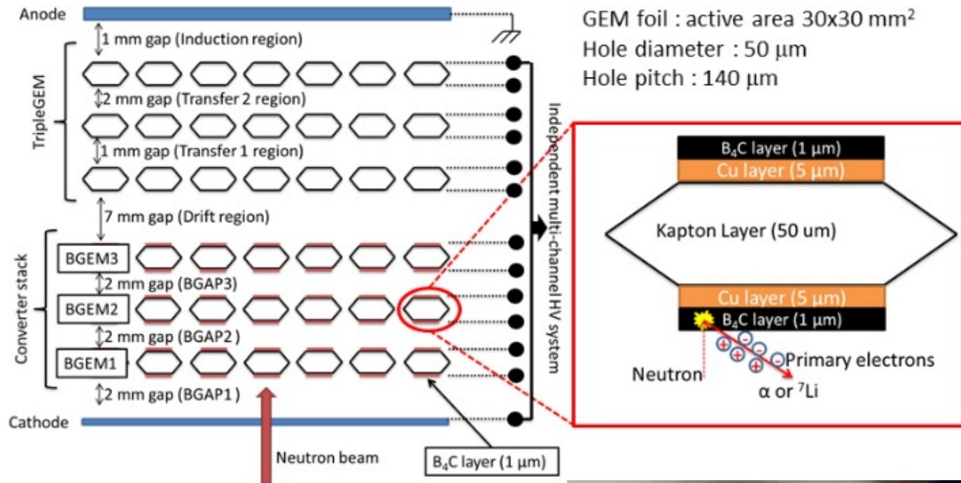
**Assembling done in Frascati of two detectors with 2- and 3-mm gap between borated gem foils**
