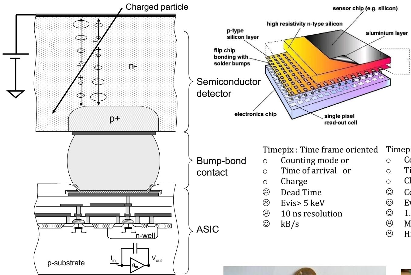
Standard CMOS can be used allowing on-pixel signal processing
