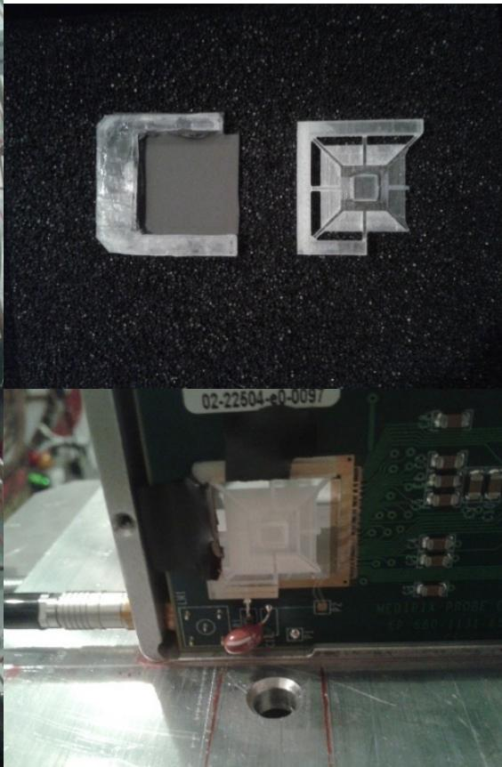
A converter can be placed on top of the silicon sensor ( $15 \times 15 \text{ mm}^2 \times 300 \text{ micron}$ )
