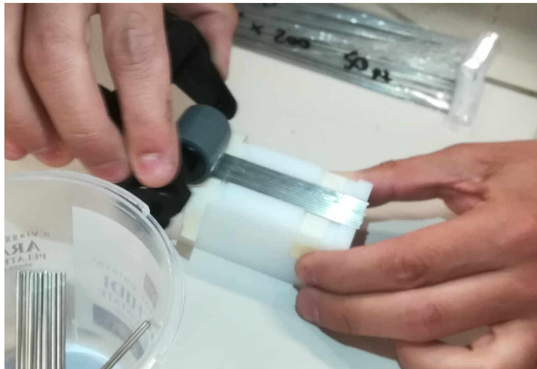
2 - glue in mixed and distributed on the tube with a small roller
