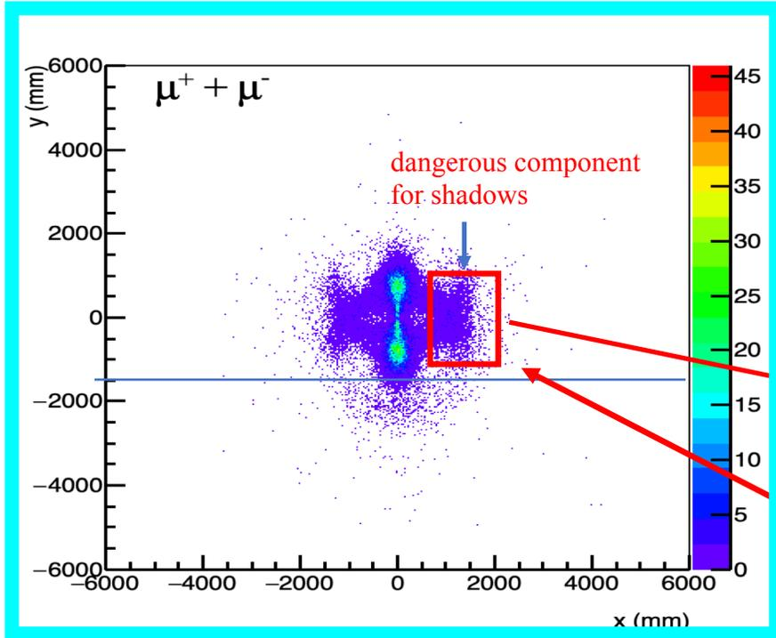
But it is made of low-p ( $< 15$  GeV) muons that can be swept away using a magnetized iron block.
