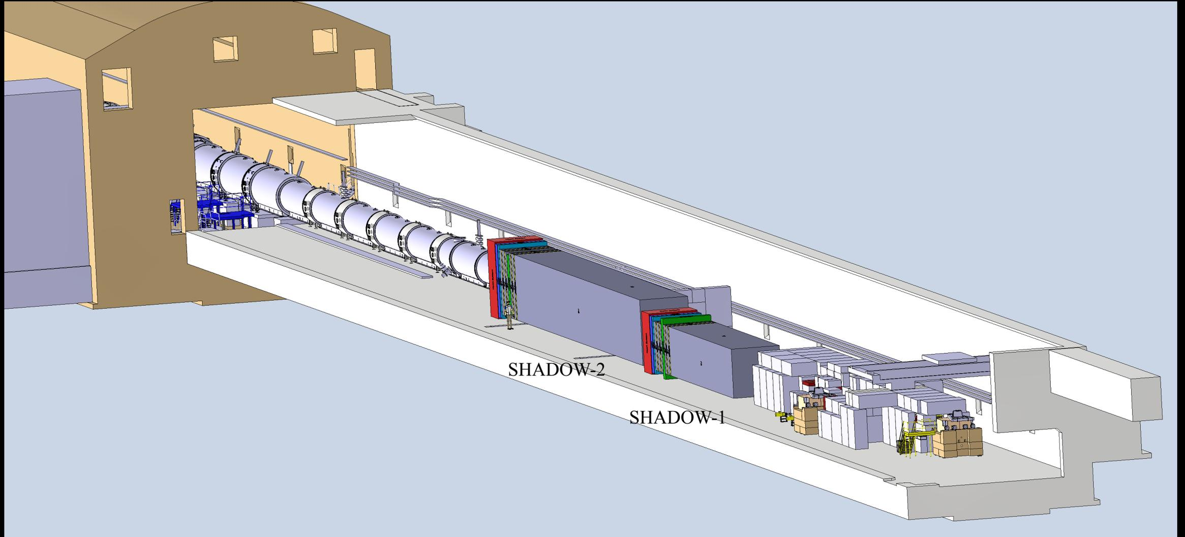
The second shadows spectrometer could have 30 m long decay volume and 3x4 m<sup>2</sup> transverse dimensions
