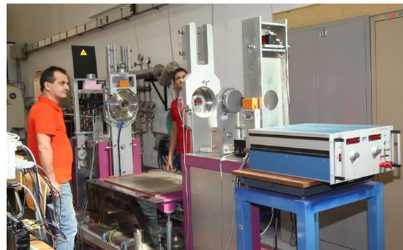
**A stretched wire bench for magnet fiducialization, integrated field measurements**
