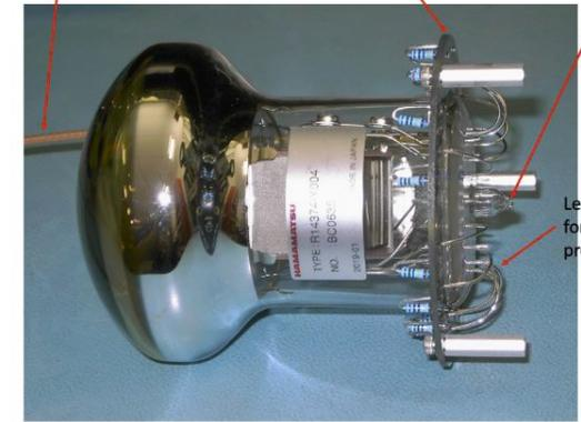
Leads bent without a form. Needs work for production scheme.
