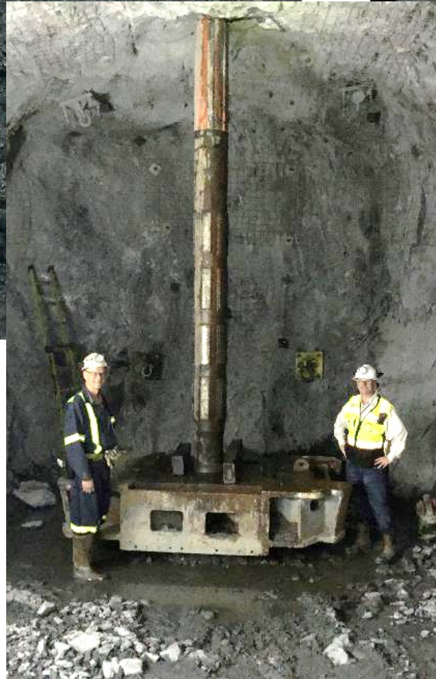
Borehole reamer (on 4850L)
