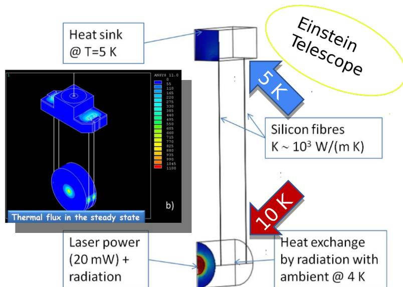
@LAE : Facility with thermal-noise limited macroscopic oscillator; ability to control thermal gradients
