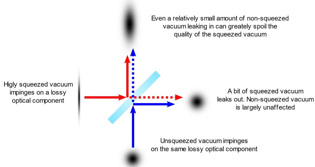
We are developing 2 technologies for sensing (and correcting) the mismatch, for the next run O4 of Advanced Virgo. The goal is to reduce to <3% the optical losses due to mode mismatch (now order 10%)
