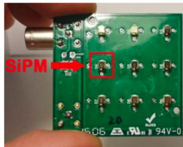
$\rightarrow$  Tested 12, 15 and 20  $\mu\text{m}$  SiPM cells up to  $\sim 2 \times 10^{11} \text{ n/cm}^2$  1 MeV-eq (max non ionizing dose for  $10^4 \text{ v}_e^{\text{CC}}$  at a 500 t v detector at  $r = 1 \text{ m}$ )
