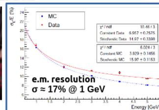
Testbeam @CERN-PS T9 beamline
