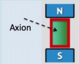
DM axions are converted into **RF photons** inside a **resonant cavity** immersed in a **strong magnetic field**
