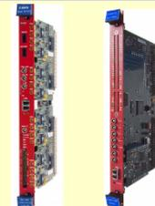
CAEN V2718 VME-PCI Optical link bridge + A3818 PCI controller
