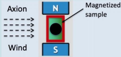
the axion DM cloud acts as an **effective RF magnetic field** on the electron spin exciting **magnetic transitions** in a magnetized sample (YIG) → **RF photons**
