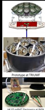
mPMT is a vessel which houses and protects an array of 19 3" PMTs:
