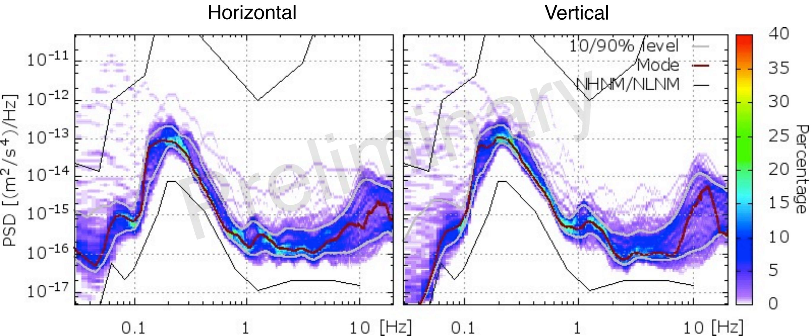
A nearby surface seismic station provided a good indication of attenuation with depth
