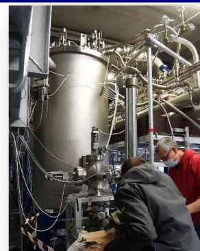
Cavity move check during vacuum pumping and cooldown
