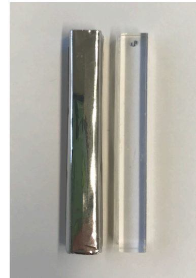
Test crystals: 40 mm length, with 5x5 mm 2 square faces
