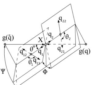
$X \rightarrow V_1V_2 \rightarrow f_{11}f_{12}f_{21}f_{22}$  $q_i \colon V_i$  momentum in X rest frame  $q_{ij} \colon f_{ij}$  momentum in  $V_i$  rest frame
