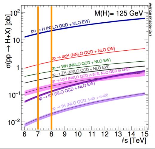
$\sqrt{s}$  Production cross section (in pb) for  $m_H = 125 \, \mathrm{GeV}$  (TeV)
