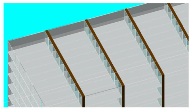
Each cell is formed by 5 layers of: 4 cm of PbF<sub>2</sub> (BIB absorber)+ SiPM+ electronics
