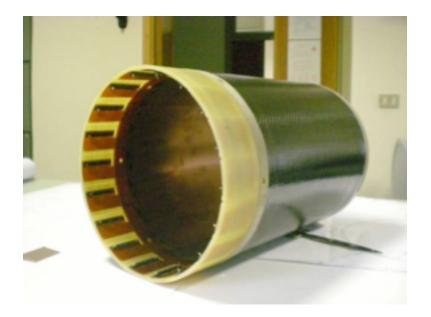
Buckling ~7.5 ton, well above the 100 kg load needed for GEM stretching.
