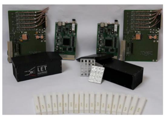
All crystals obtained by SICCAS (Shangai), QA done @Rome1 3x3 mm<sup>2</sup> SIPM from Hamamatsu, FEE from SELF (LNF)
