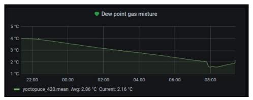
I adjusted the dry mixture to 7.2 l/h and the Dew point was back to the acceptable values +- 4°C
