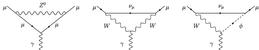
$$a_\mu^{\text{EW}}(\text{1-loop}) = \frac{5G_\mu m_\mu^2}{24\sqrt{2}\pi^2} \left[ 1 + \frac{1}{5} (1 - 4 \sin^2 \theta_W)^2 + O\left(\frac{m_\mu^2}{M_{Z,W,H}^2}\right) \right] \approx 195 \times 10^{-11}$$
