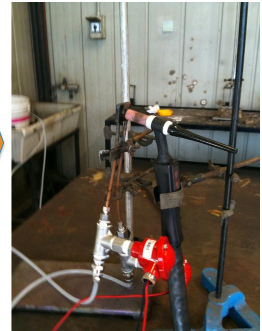
Preliminary Tests done depositing a thin Indium layer instead of Lithium.
