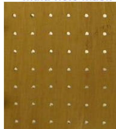
reconstruction of the hole mask put in front of the detector for calibration
