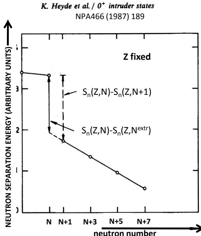
Fig. 3. Outline of a graphical method in order to obtain the unperturbed particle-hole energy in a given closed shell nucleus  $A(Z, N)$ , where  $Z(N)$  denote the proton (neutron) number of the shell closure, starting from empirical proton separation energies  $S_p$ . The dashed line denotes the standard prescription, the full line the new prescription.  $Z^{\text{extr}}$  denotes the extrapolated value for the proton separation energy from above the shell closure.
