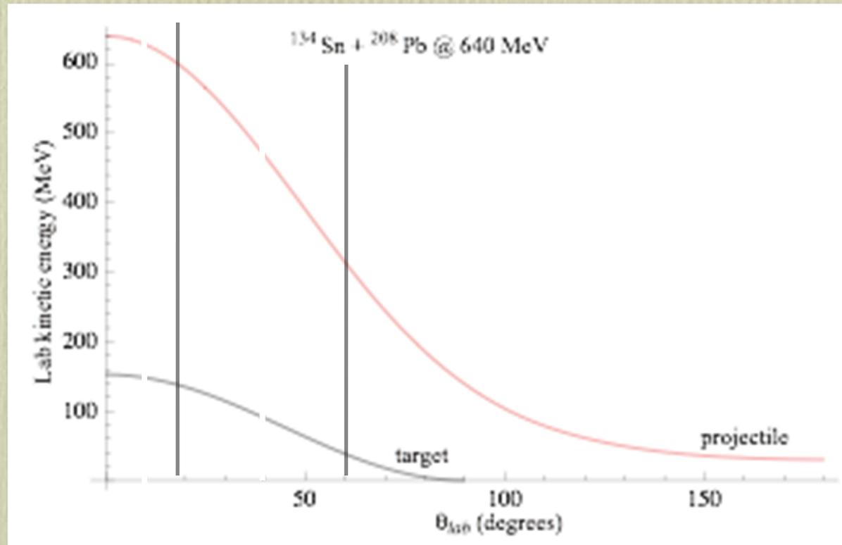
With the Si detector mounted at 5 cm distance from the target  $\longrightarrow$   $\theta$  coverage: 18 to 60 degrees
