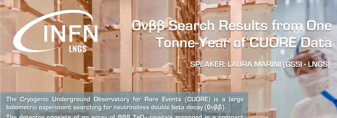
The detector consists of an array of 988 TeO<sub>2</sub> crystals arranged in a compact structure of 19 towers, hosted in the biggest cryostat ever built to operate at 10mK.
