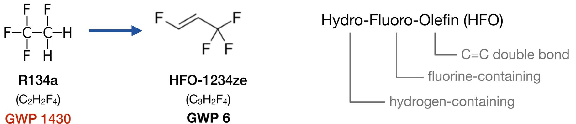
*New eco-friendly liquids/gases have been developed for industry as refrigerants and HV insulating medium... not straightforward for RPC operation*
