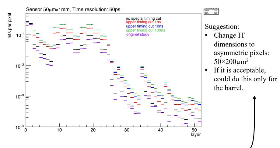
• IT is layers 24-27: For the IT barrel, opening cut to 1ns would lead to 4-8% occupancy for barrel. What to do?
