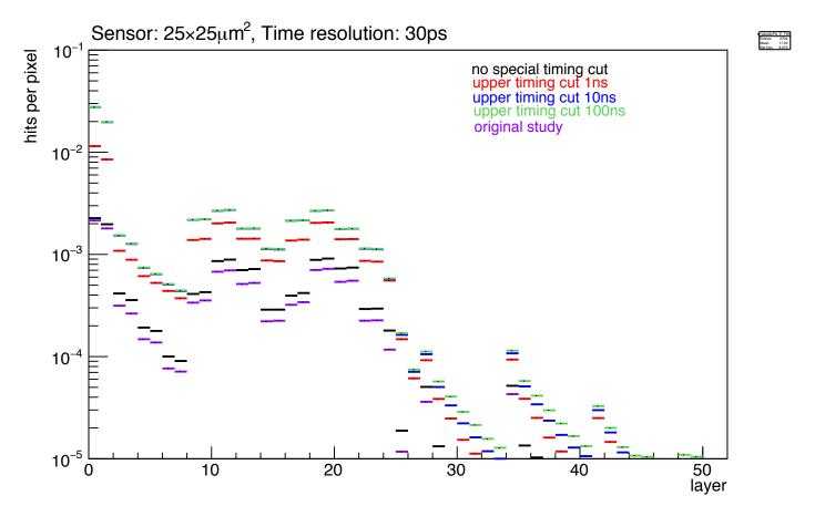
• For  $25 \times 25 \mu m^2$  and  $\sigma_t = 30 ps$ , opening up upper cut would work, especially for all but two innermost layers.
