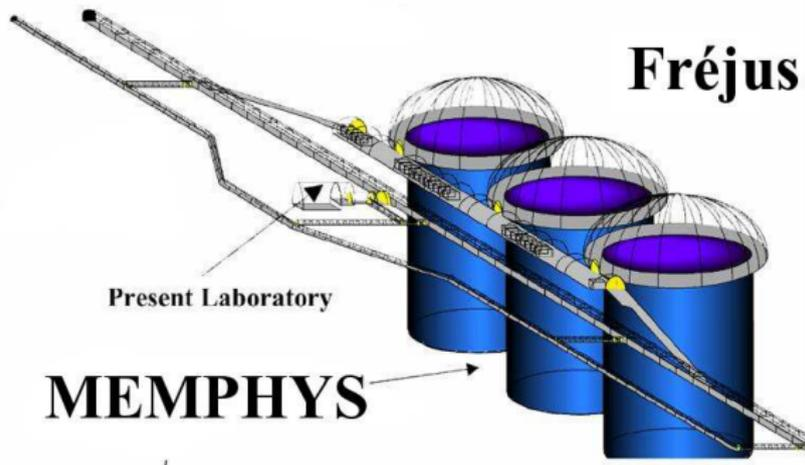
In the middle of the Fréjus tunnel at a depth of 4800 m.w.e excavate three shafts of about 250,000 m<sup>3</sup> each ( $\Phi = 65$  m, full height=80 m). 440 kton fiducial volume
