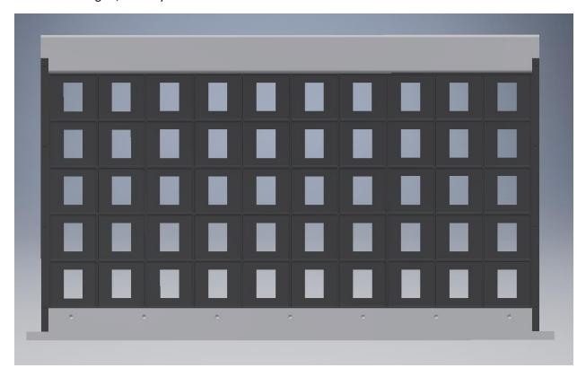
PDs will be housed on the back face of the crystal, so the wrapping material should have the same aperture as the array structure.
