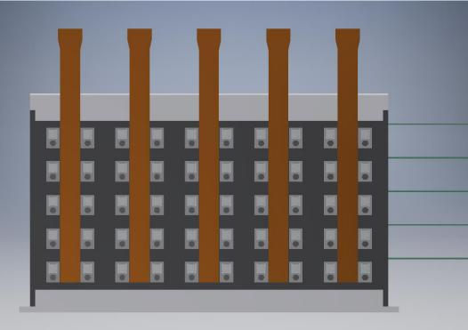
The array structure has an aperture in the centre of each cell which should contain the multipackage with come margins, let's say 20x13.5 mm.
