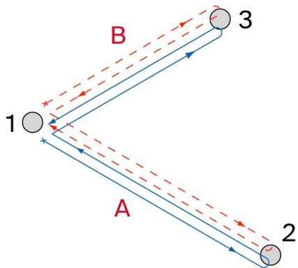
Time Delay Interferometry: Combine phase measurements retarded in time in such a way that laser frequency noise is killed
