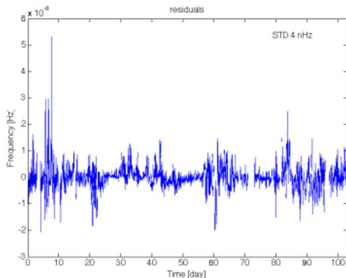
$\omega_{local}$  is instrumental, when the monument tilts the mechanical structure of GINGERINO rotates. Improvement of the heterolithic mechanical design required.
