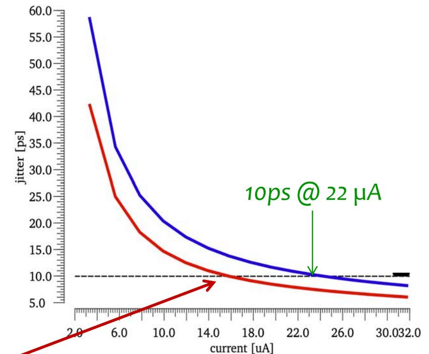
Time jitter vs current consumption of the CSA stage (CMOS 28-nm). Red curve: **schematic simulation**. Blue curve: **post-layout simulation after parasitics extraction**.
