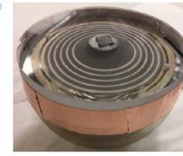
Hybrid photosensor: ABALONE; left (DARWIN R&D with SiPM); right: NIM 954, 2020
