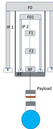
A seismic isolation system adopting a nested, double inverted pendulum could permit large improvement in seismic isolation keeping total suspension length comparable with the AdV superattenuator.
