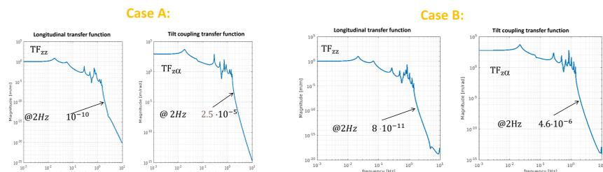
Just increasing the length of the suspension the tilt coupling @2Hz is reduced by a factor of 5.5.
