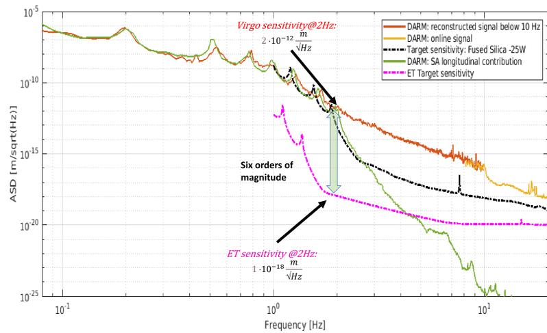
To achieve the attenuation value of  $10^{-18} \text{m/sqrt(Hz)}$  at few Hz, the suspensions of the optical components must be upgraded with respect to the 2<sup>nd</sup> generation ones, in order to improve seismic attenuation in low frequency and reduce as much as possible the frequency of mechanical resonances below the detection band.
