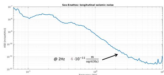
At the moment, there is no direct measurement of tilt ground but it is possible to estimate a lower limit by using the following empirical formula:  $\alpha_0 = \frac{g}{v} \cdot x_0$
