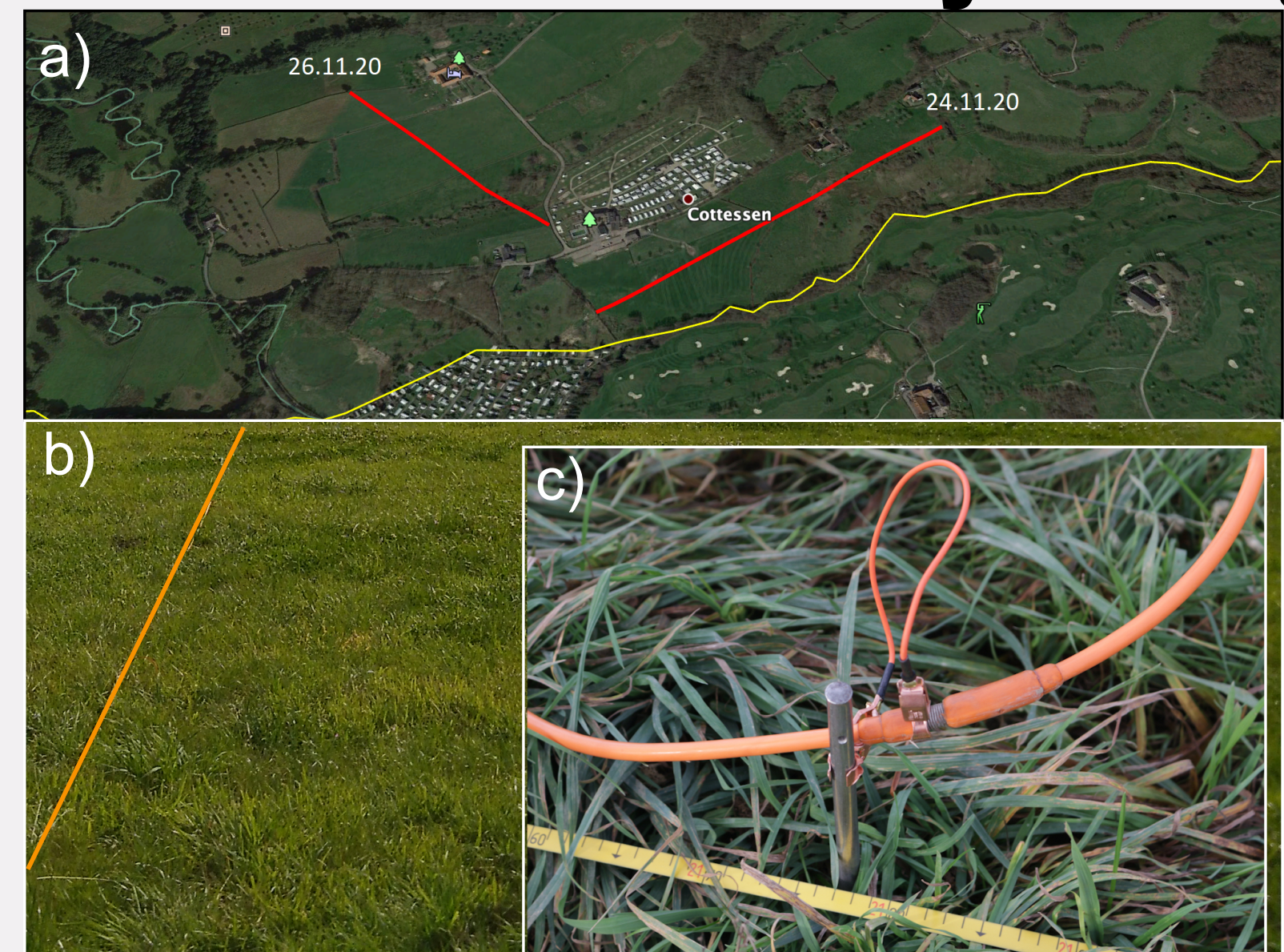
Fig. 6: a) Map showing ERT profile lines around the village of Cottessen. b) ERT profile line on a field (orange line). c) Electrode to measure the resistivity.
