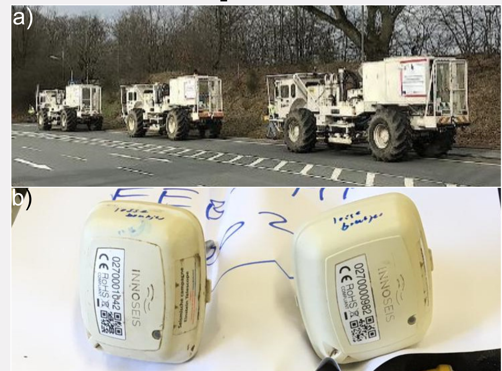
Fig. 4: a) Active seismic survey using vibro-seis truck to generate energy. This energy input allows mapping to a depth of several kilometres b) Battery-operated sensors recording any occurring seismic signal.
