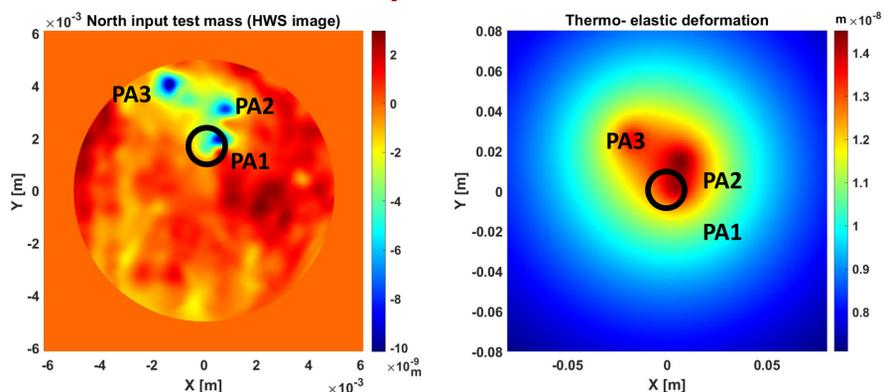
On the left: Wavefront map measured by the HWS-DET probing the NI test mass. WF has been acquired two minutes after the ITF is locked at dark fringe. This is the first in which it is possible to see the three point absorbers. On the right: The simulated thermo-elastic deformation due to the points, based on the analysis of the HWS image. The Gaussian weighted RMS value of the thermo-elastic map is  $1.50 \cdot 10^{-9}m$ . The center of the mirrors is in the regions inside the black circles.
