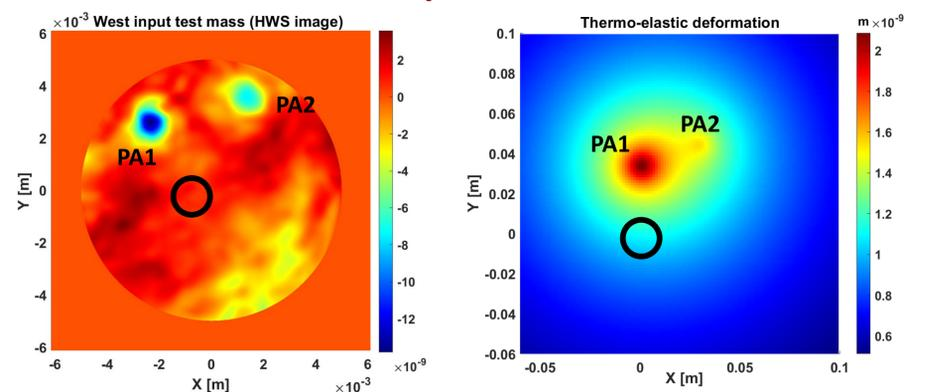
On the left: Wavefront map measured by the HWS-INJ probing the WI test mass. WF has been acquired one minute after the ITF is locked at dark fringe. This is the first in which it is possible to see the two point absorbers. On the right: The simulated thermo-elastic deformation due to the points, based on the analysis of the HWS image. The Gaussian weighted RMS value of the thermo-elastic map is  $2.6 \cdot 10^{-10}m$ . The center of the mirrors is in the regions inside the black circles.
