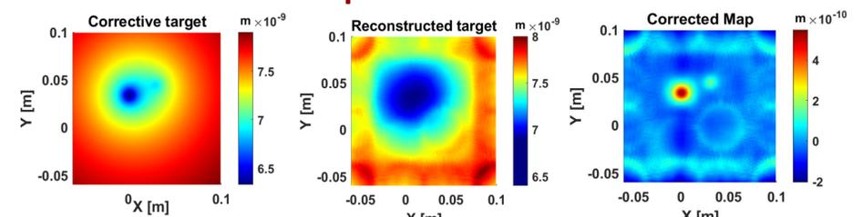
On the left: The WI corrective target to be reproduced. In the center: The reconstructed target by 144 actuators. On the right: The corrected map obtained by the sum of the initial thermo-elastic deformation and the reconstructed target. The Gaussian weighted RMS before the correction is  $2.6 \cdot 10^{-10}m$ , after the correction the value is  $7.7 \cdot 10^{-11}m$ .
