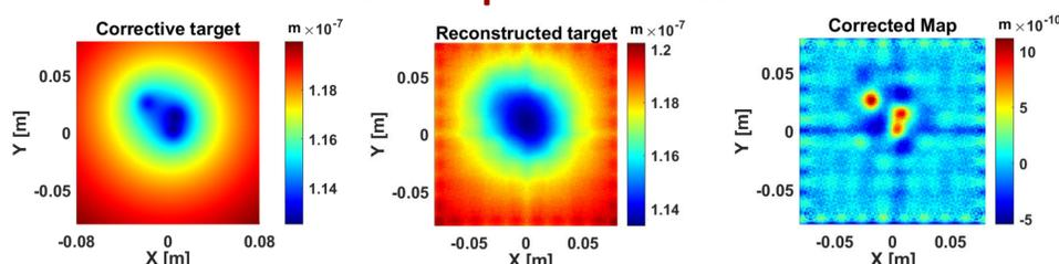
On the left: The NI corrective target to be reproduced. In the center: The reconstructed target by 100 actuators. On the right: The corrected map obtained by the sum of the initial thermo-elastic deformation and the reconstructed target. The Gaussian weighted RMS before the correction is  $1.50 \cdot 10^{-9}m$ , after the correction the value is  $2.42 \cdot 10^{-10}m$ .
