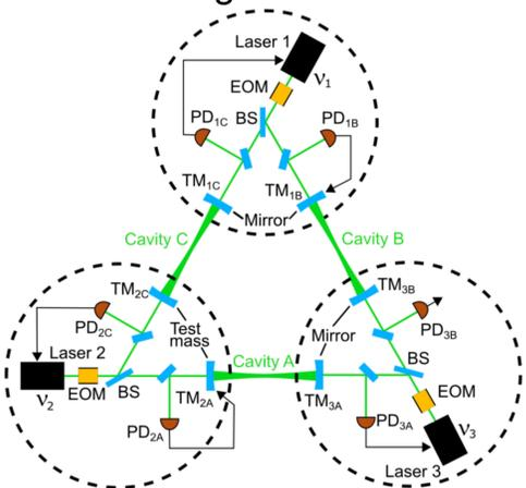
Fig. 1: Schematic view of the DPDFPI considered for DECIGO.
