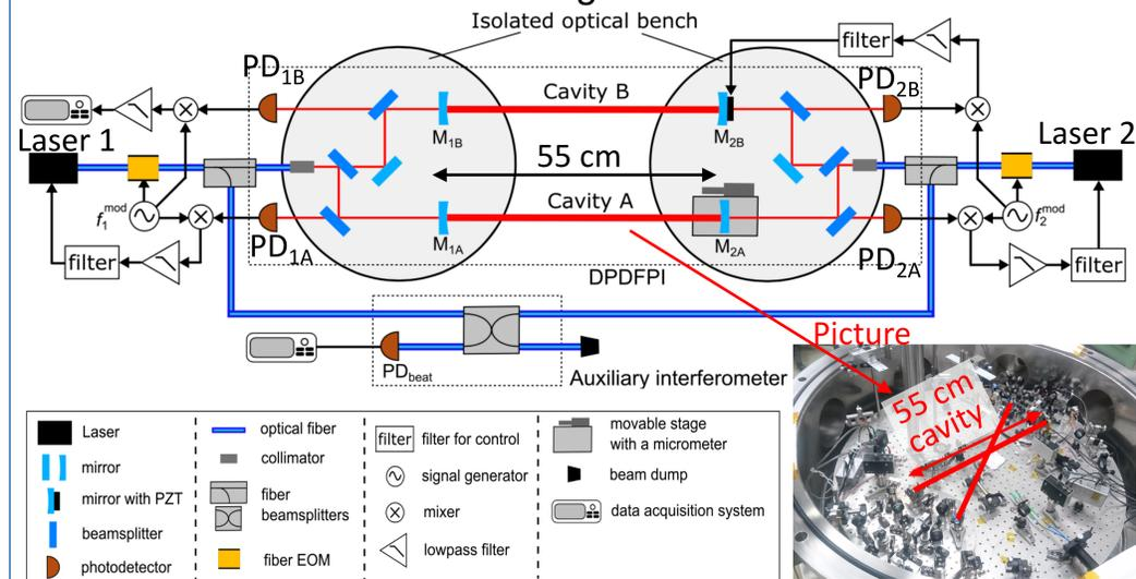
Fig. 3: Schematic of the DPDFPI experiment. The free-space interferometer on the isolated optical bench is the DPDFPI. The fiber-based interferometer is the auxiliary interferometer for the cavity absolute length measurement.
