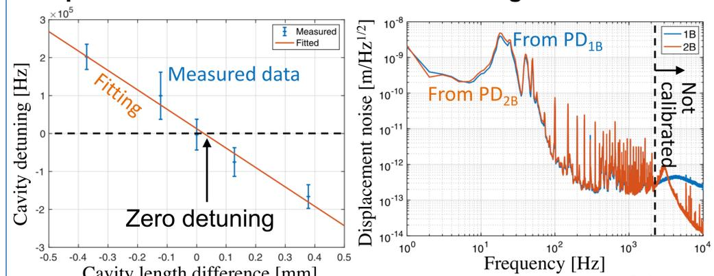
Fig. 4: Measured cavity detuning.
