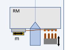
Moving mass m = 20g on the TM, m could be optimized to improve range or tolerances
