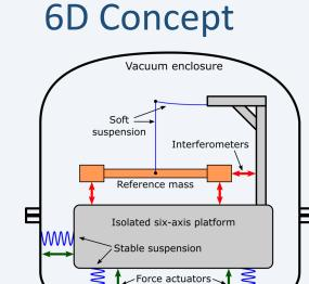
Impose the inertial stability of the reference mass on the isolated platform using active feedback.
