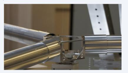
Fused silica suspension is tested for a smaller mass (up to 700g). Full Reference mass suspension is planned soon.
