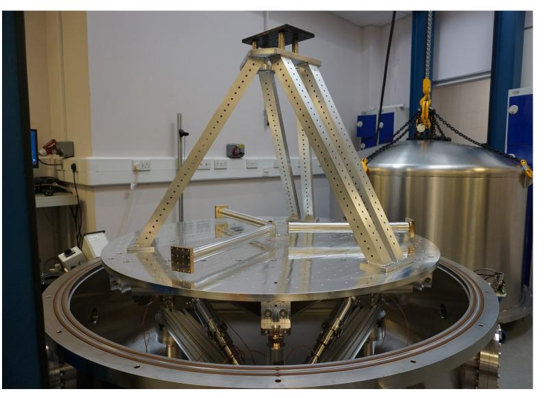
Actuated platform is recently installed in the vacuum chamber.
