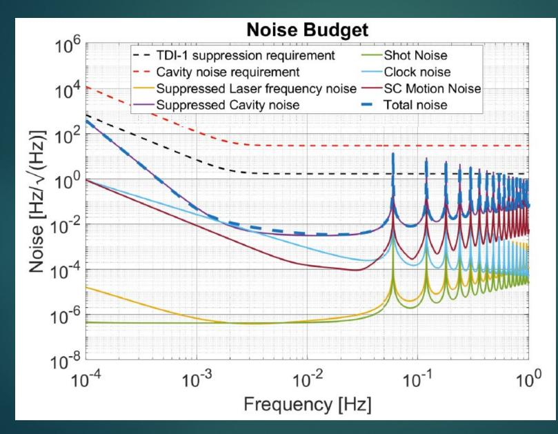
Suppression requirement for LISA can be realized with this controller setup and can perform better than the cavity alone.
