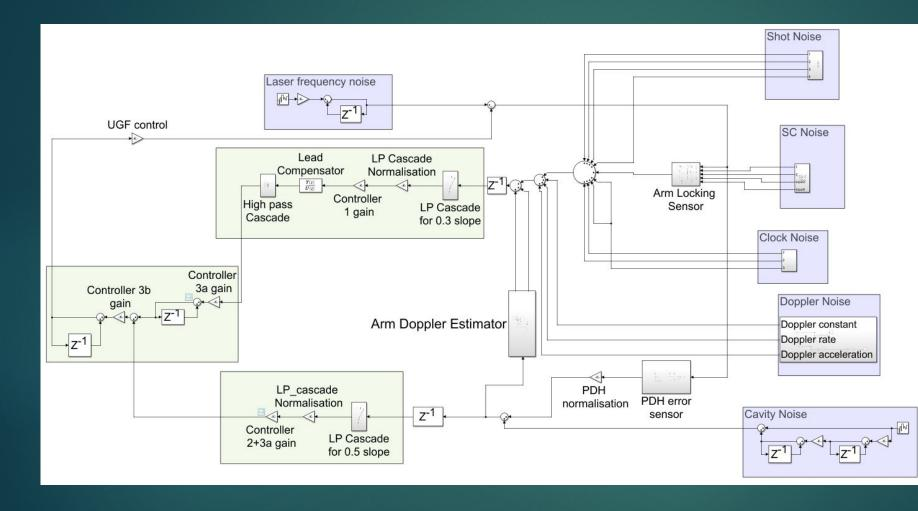
UGF is at 500 Hz, with the sampling frequency at 10 kHz.
