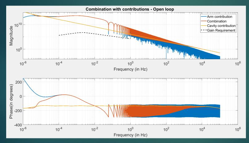
Unity Gain Frequency ~10 kHz Phase Margin at UGF ~  $30^{\circ}$ Phase margin at lower gain crossover point ~ $52^{\circ}$ Arm dominant from 10  $\mu$ Hz to 2 kHz.
