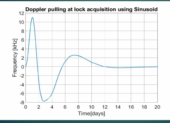
Cavity linewidth ~ 200 kHz Doppler requirement < 15 kHz
