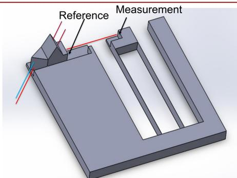
Figure 1: Resonator and interferometer combination design
