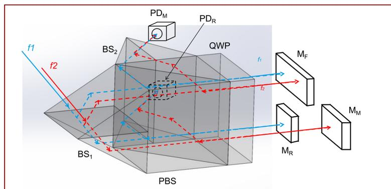
Figure 2: Compact quasi-monolithic heterodyne laser interferometer design
