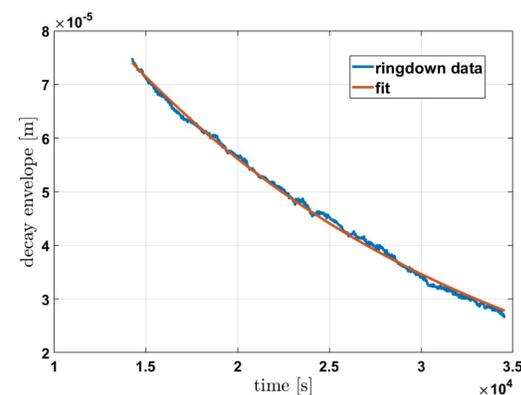
Figure 5: A 12-hour ringdown measurement at 1 mTorr. From the exponential fit, we find a mechanical quality factor of  $2.45 \times 10^5$ .
