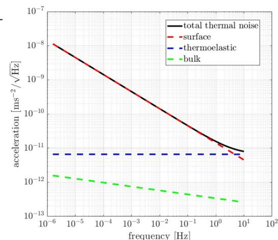
Figure 4: Estimated acceleration sensitivities for these resonators are on the order of  $10^{-11} \text{ ms}^{-2}/\sqrt{\text{Hz}}$ <sup>[1]</sup>
