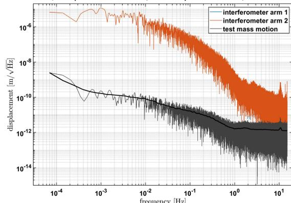
Figure 3: Most recent spectral density of the benchtop interferometer prototype at atmospheric pressure
