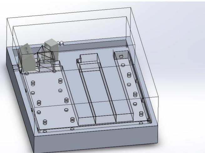
Figure 6: Preliminary mount design to hold the interferometer, resonator, fiber injectors, and photodetectors.
