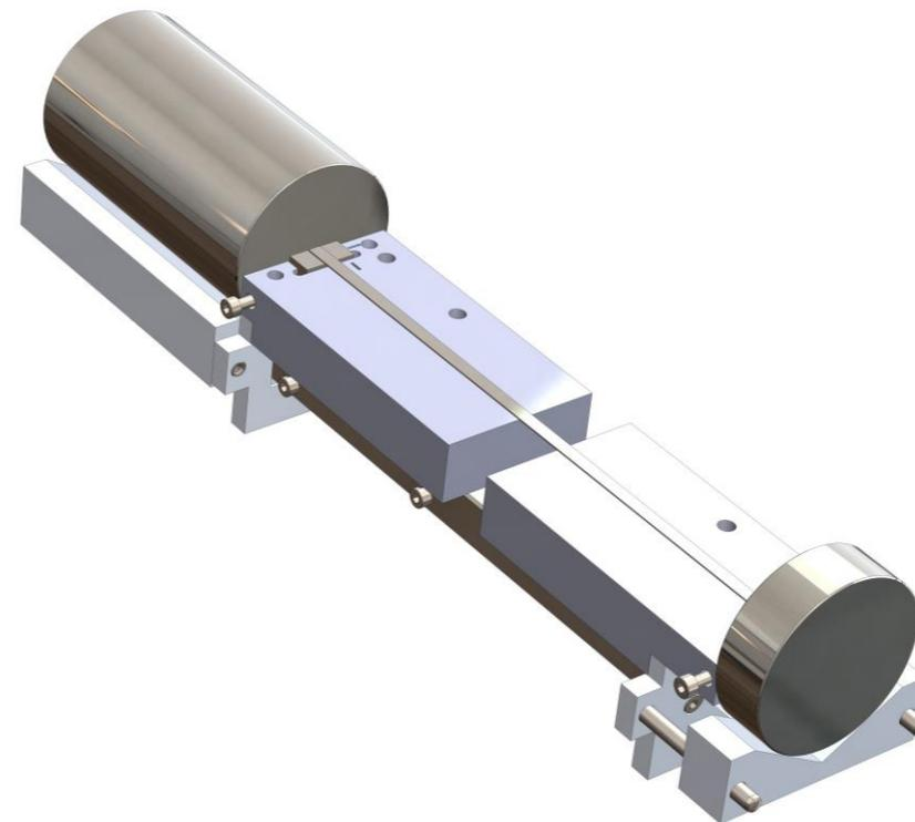
Hydroxyl catalysis bonding jig
