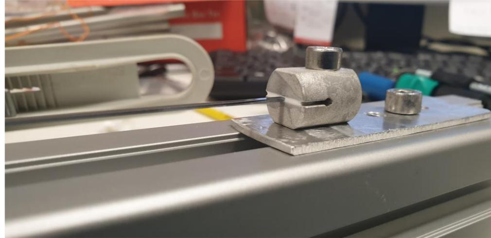
Aluminium fuse end, glue and silicon
