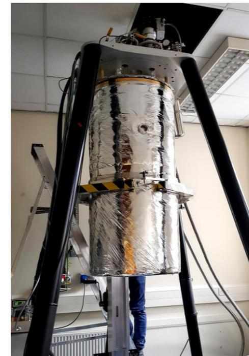
Closing up cryostat – 50K shield shown with lifting pincers
