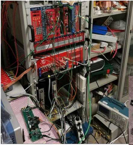
The local modular fanout is used to provide FCS signals (clock and trigger) to the 2 GEMROC modules used in the setup
