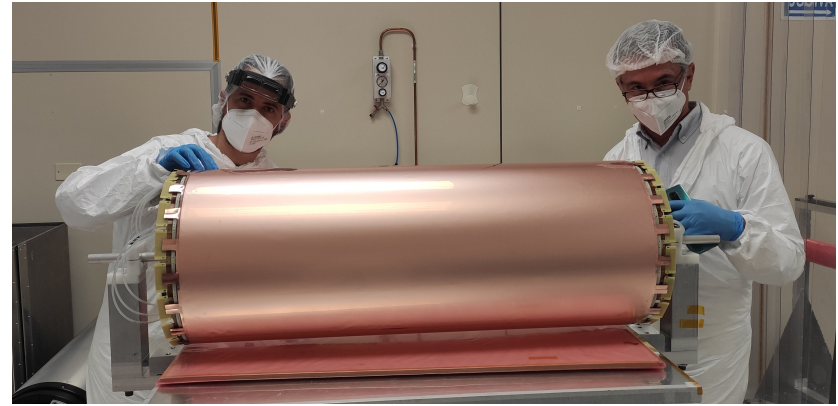
Faraday Cage finally covering L3
