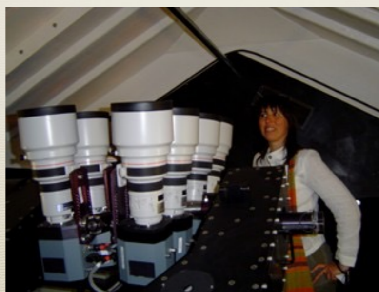
The NGTS 20cm telescopes on their mounts in the enclosure at ESO Paranal (Credit:ESO/R. West)
