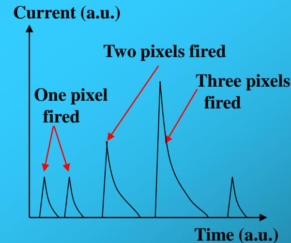
A single GM-APD gives no information about light intensity  $\Rightarrow$  in a SiPM the output charge is proportional to the number of triggered cells, that is (for PDE = 1) the number of photons
