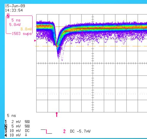
Bandwidth from DC to 700 MHz, gain 16.3 dB
