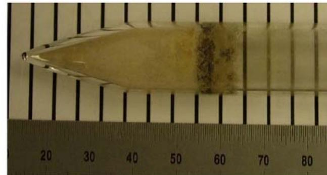
Fig. 1. A 1 cm in diameter Ba<sub>2</sub>CsI<sub>5</sub>:Eu<sup>2+</sup> shown as-grown in a sealed quartz ampoule.
