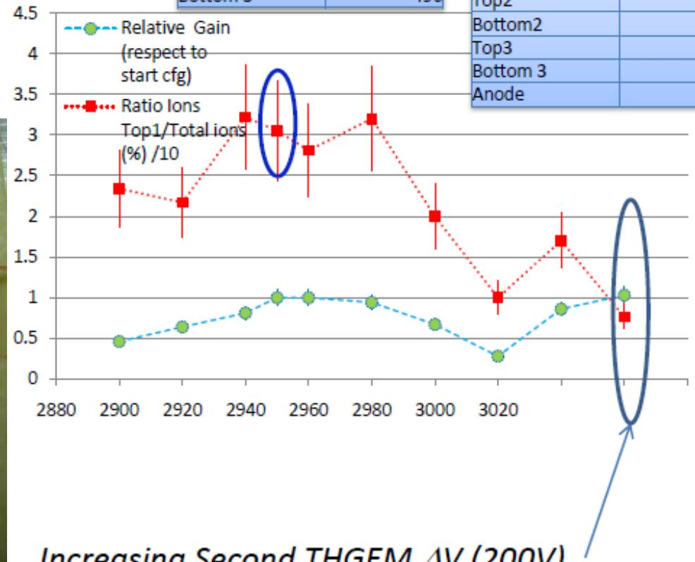
Reduction by a factor 4 of the ion feed-back without gain losses
