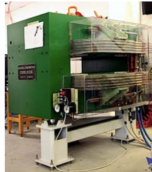
Dipole magnet (CERN TE/NSC-MNC)
