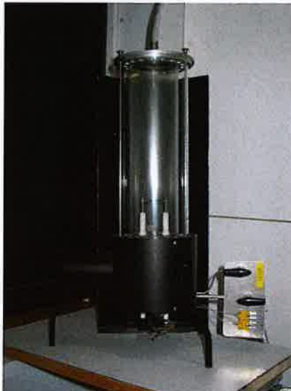
figure 1: glass tube for the flammability test according to ISO 10156
