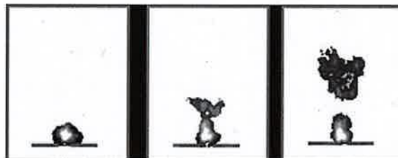
figure 2: illustration of a flame detachment with flame propagation over a distance of at least 100 mm as criterion for flammability
