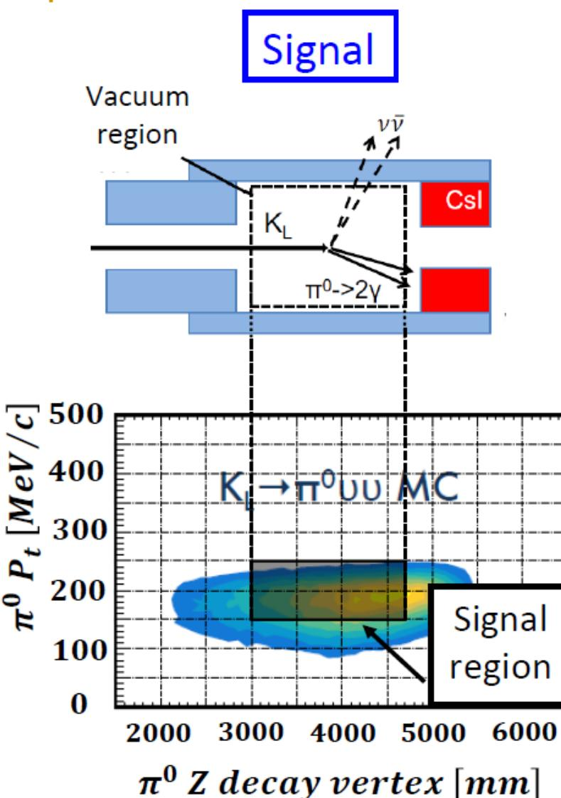
Hermetic detector and efficient photon detection
